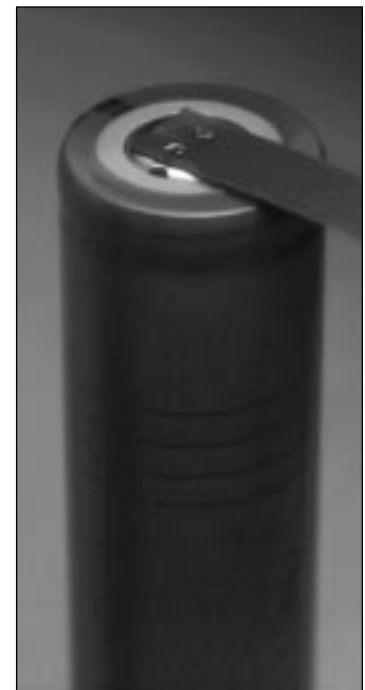
Electro-Plated Nickel Plated Steel tab to 18650 Li-Ion cell.
