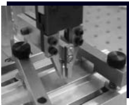
FIGURE 2. Parts handling represents a challenge for both tooling and automation. A gripper tool is used to secure and position the ferrule and clip as a subassembly.
