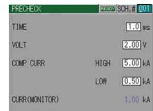
Pre-Check of resistance prior to welding
