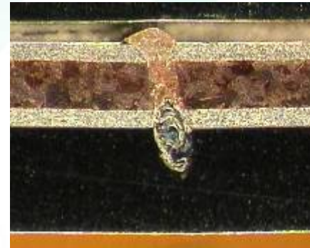
0.012" thick nickel clad copper to 0.015" thick steel
