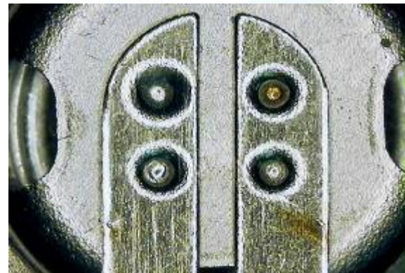
0.012" thick nickel clad copper tab to steel terminal
